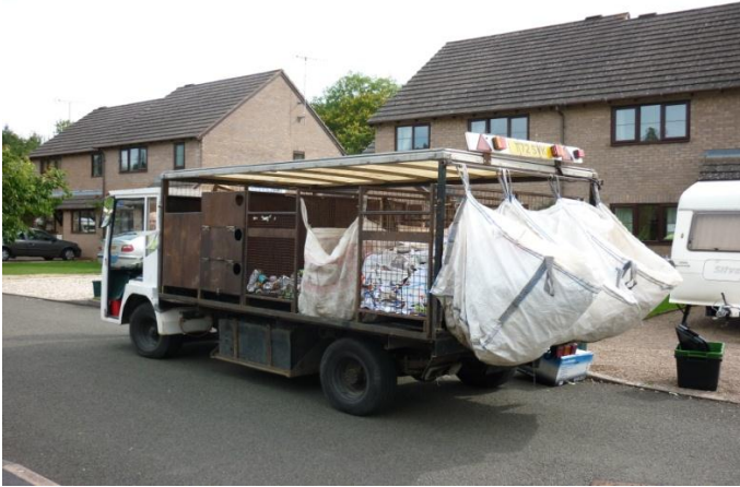
Figure 6.2.1 Collection vehicle used in the Presteigne. Food waste and dry recyclables are collected on the same vehicle. The food waste pod is the stillage closest to the drivers cab (Photo courtesy of Cwm Harry Land Trust)
