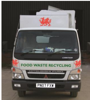
Figure 6.3.1 The 7.5 tonne purpose built 'pod and bin lift' vehicle operated by Cwm Harry Land Trust (Photographs courtesy of Cwm Harry Land Trust)
