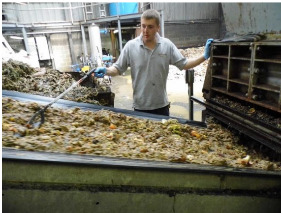
a) removal of biodegradable bag (by hand) from the shredded food waste on the belt
